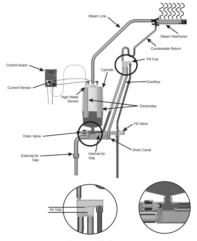
Figure 29: Humidifier Schematic
