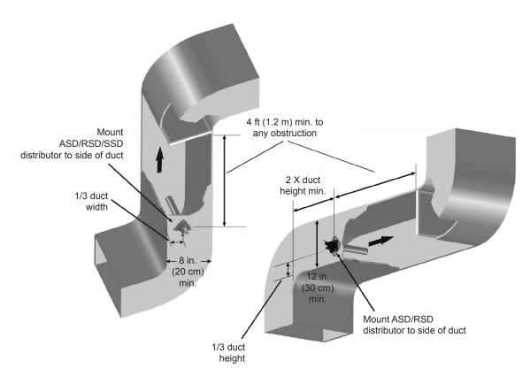
Figure 8: RH2+ Duct RSD10, ASD10 and SSD Distributor Installation
