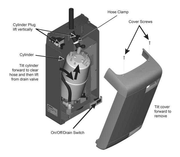
Figure 34: Cylinder Removal
