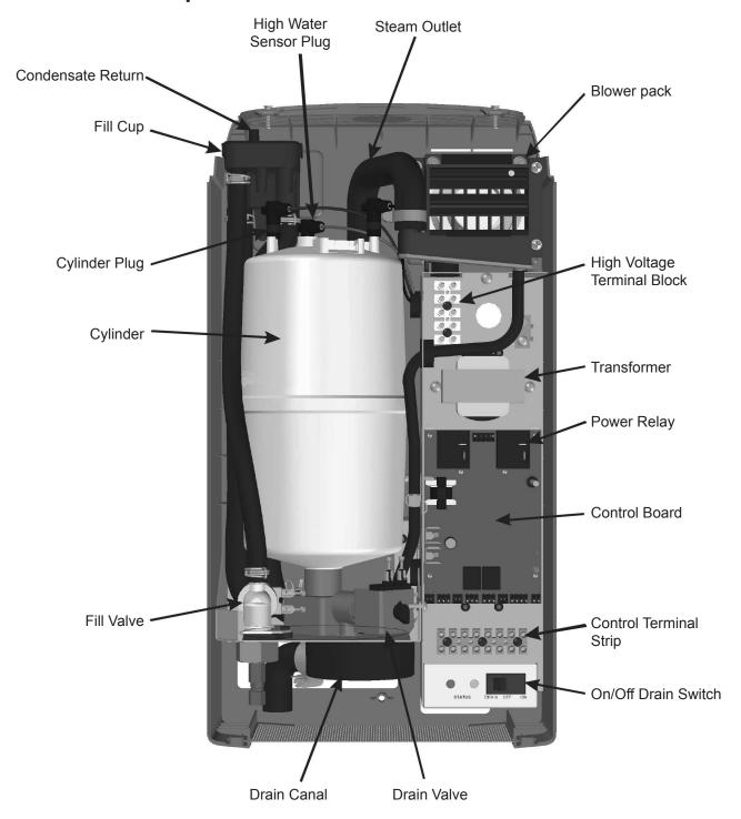
Figure 28: RH2+ Humidifier Components
