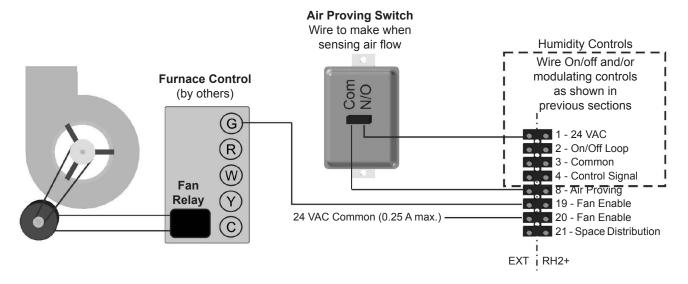
Figure 22: RH2+ Fan Enable Wiring
