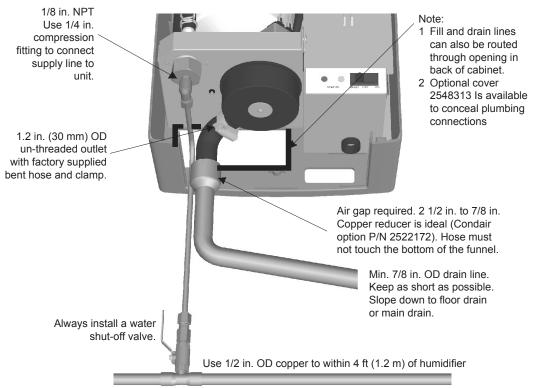
\* Pipe and water shut-off valve not supplied by Condair.
