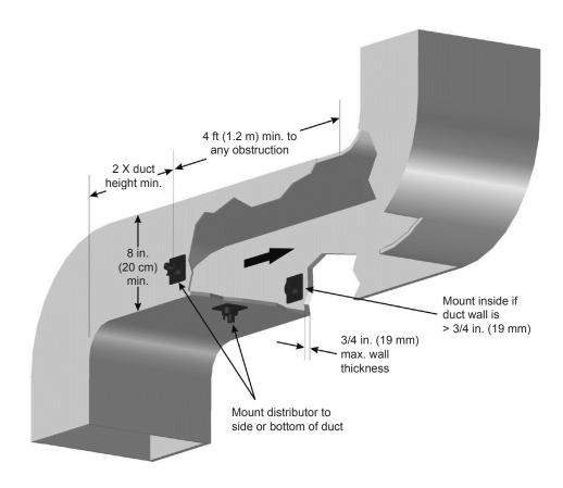
Figure 7: RH2+ Duct Nozzle Distributor Installation
