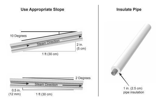
Figure 10: Main Steam Line Requirements
