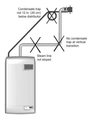
Figure 14: Common Steam Line Errors
