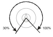
Figure 32: Capacity Potentiometer Adjustment
