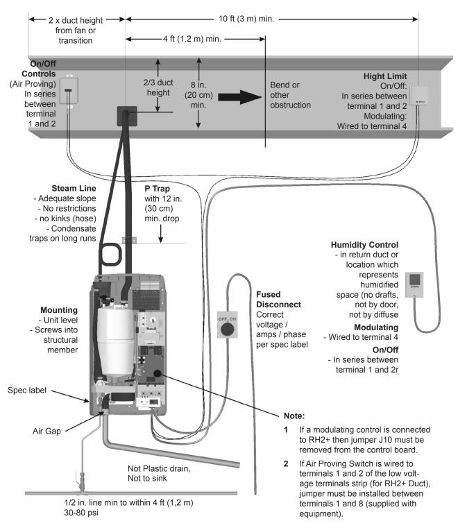
Figure 25: Installation Check
