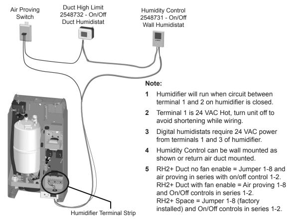
Figure 18: On/Off Controls
