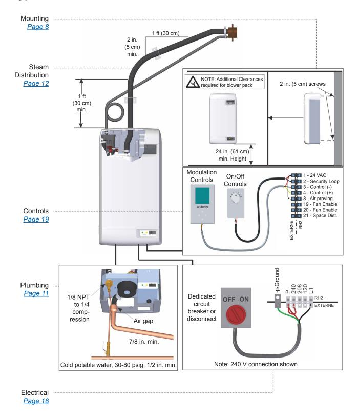
Figure 3: Typical Humidifier Installation
