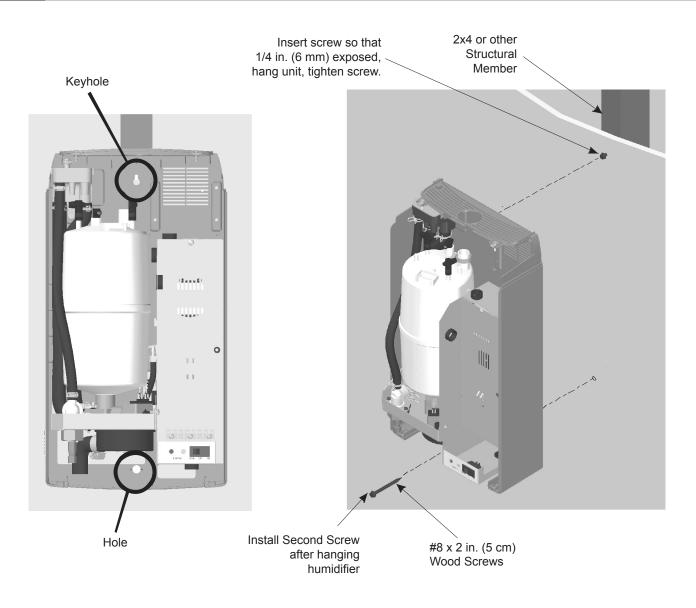
Figure 5: Mounting With Keyholes
