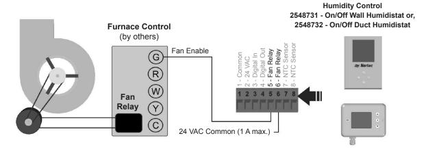
Figure 23: Digital On/Off Humidistat Fan Enable
