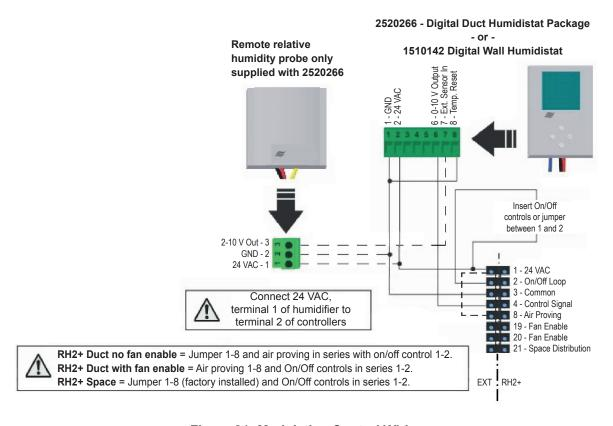
Figure 21: Modulating Control Wiring
