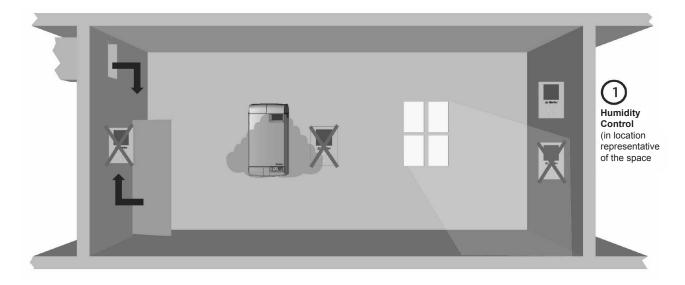
Figure 17: Control Location (In-Space Humidification)
