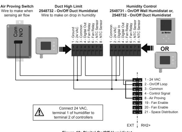
Figure 19: Digital On/Off Humidistat
