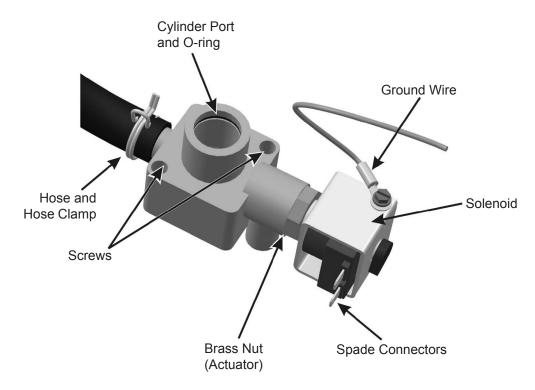
Figure 35: Drain Valve
