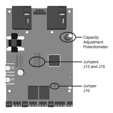
Figure 31: RH2+ Control Board Jumpers
