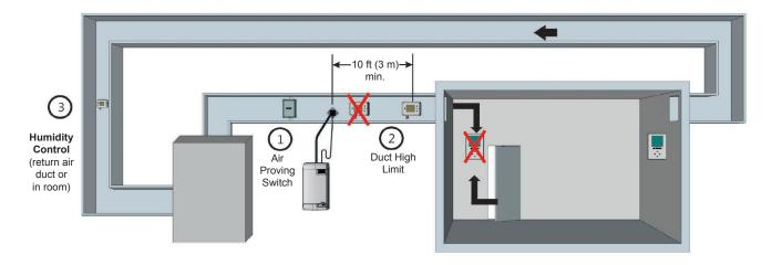
Figure 16: Control Location (Duct Humidification)
