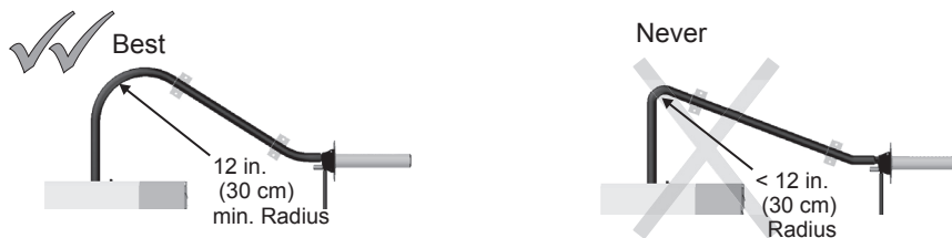
Figure 4: Minimum bend radius in steam lines.
