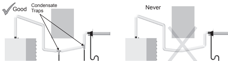
Figure 9: Condensate trap installation at low points in line and at horizontal to vertical transitions.
