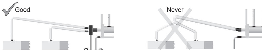
Figure 6: Connecting multiple steam lines to a single distributor.
