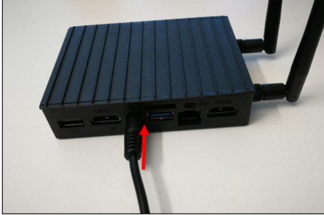
Fig. 39: Connecting the gateway to the power supply
