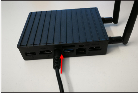
Fig. 36: Connecting the gateway to the power supply
