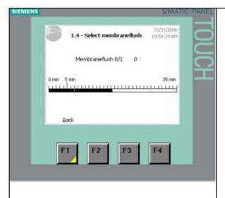
\*From the basic setup screen 1.0 press F1 for membrane flush.
