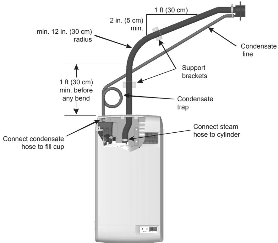
**Figure 11: Steam Distributor Above Humidifier (using Condair hose)**
