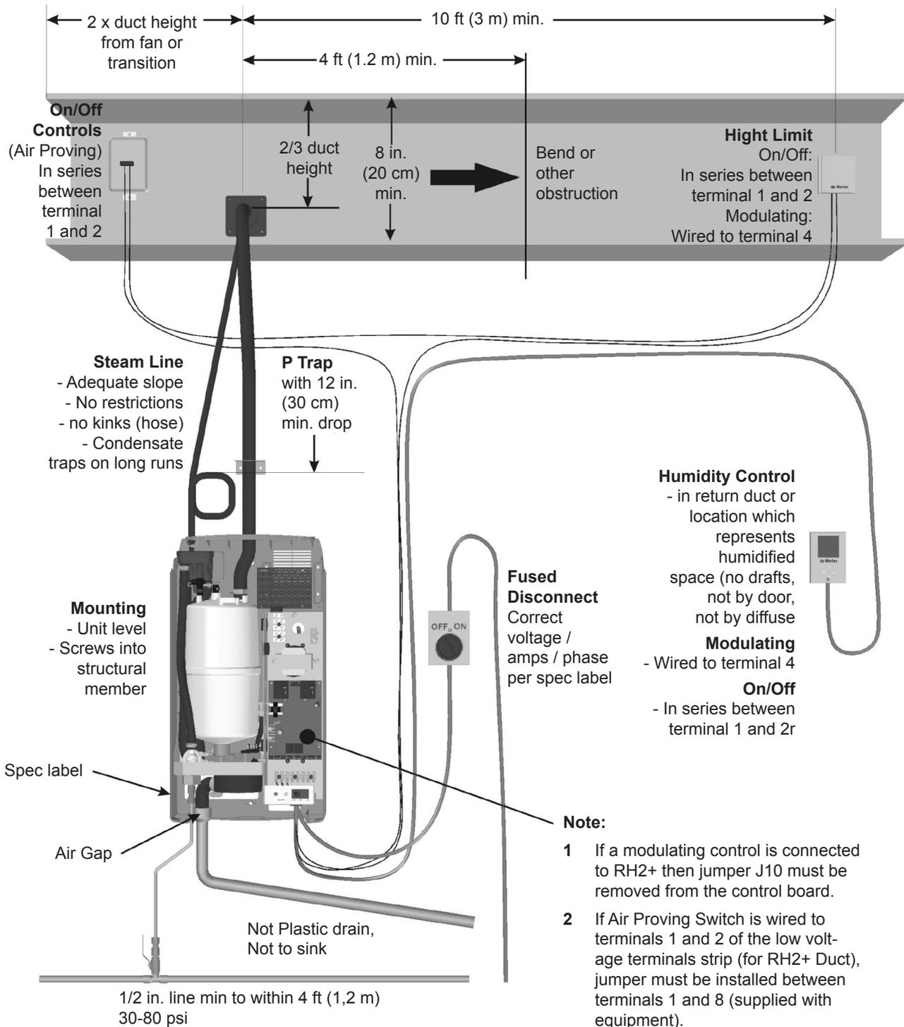
**Figure 25: Installation Check**
