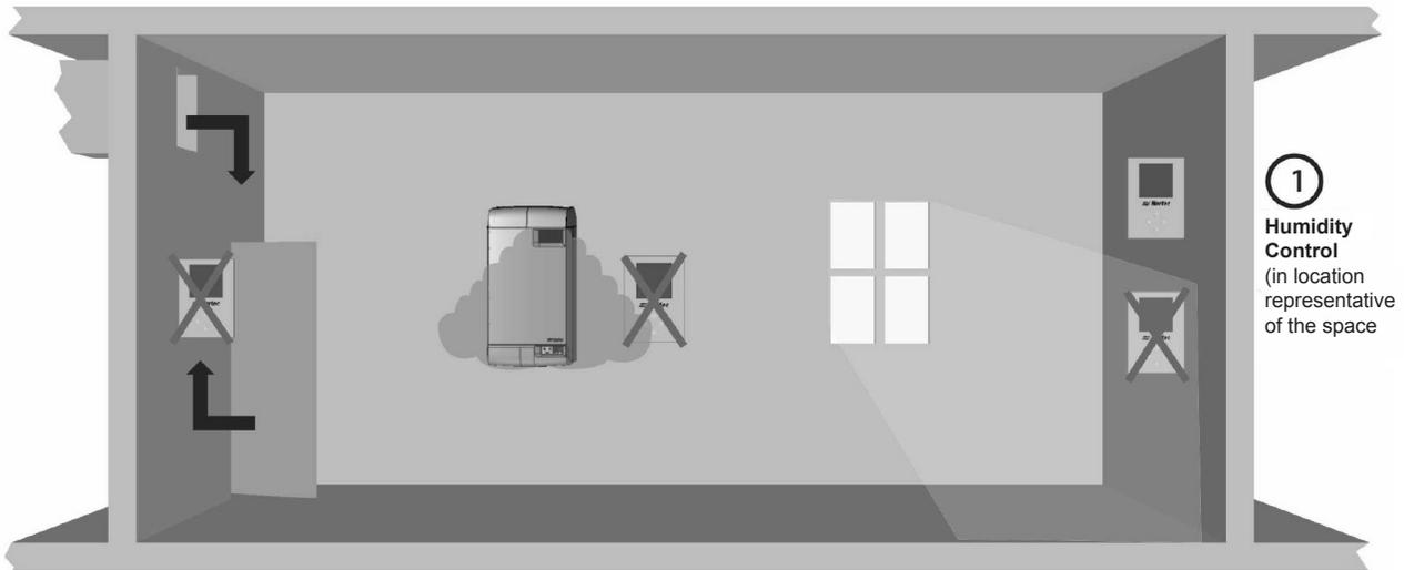
**Figure 17: Control Location (In-Space Humidification)**
