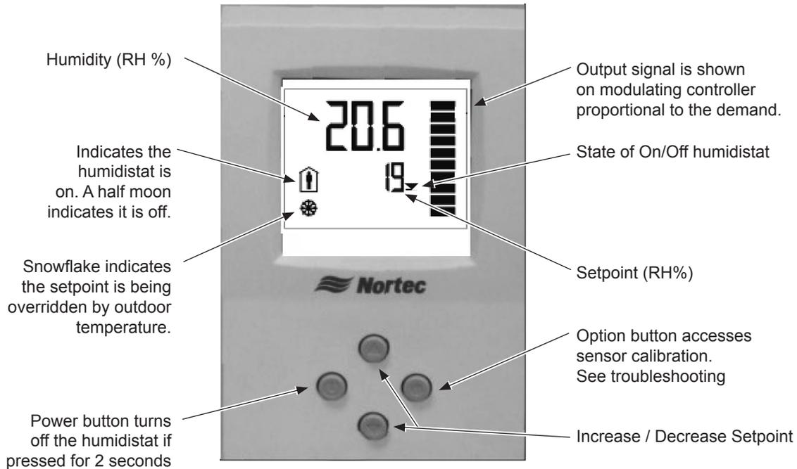
**Figure 26: Modulating and On/Off Digital Control Operation**
