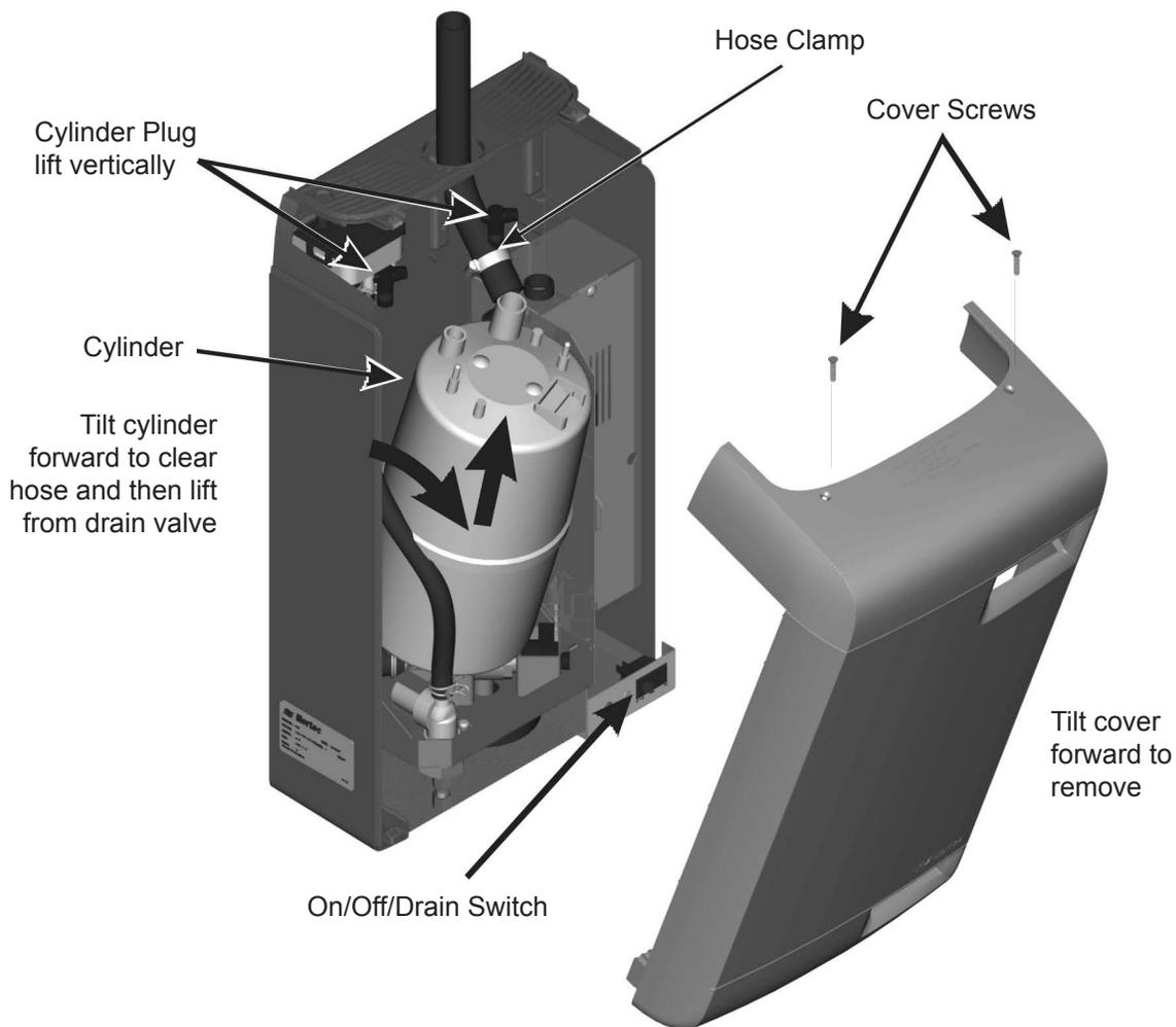
**Figure 34: Cylinder Removal**
