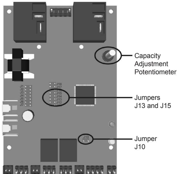
Figure 31: RH2+ Control Board Jumpers
