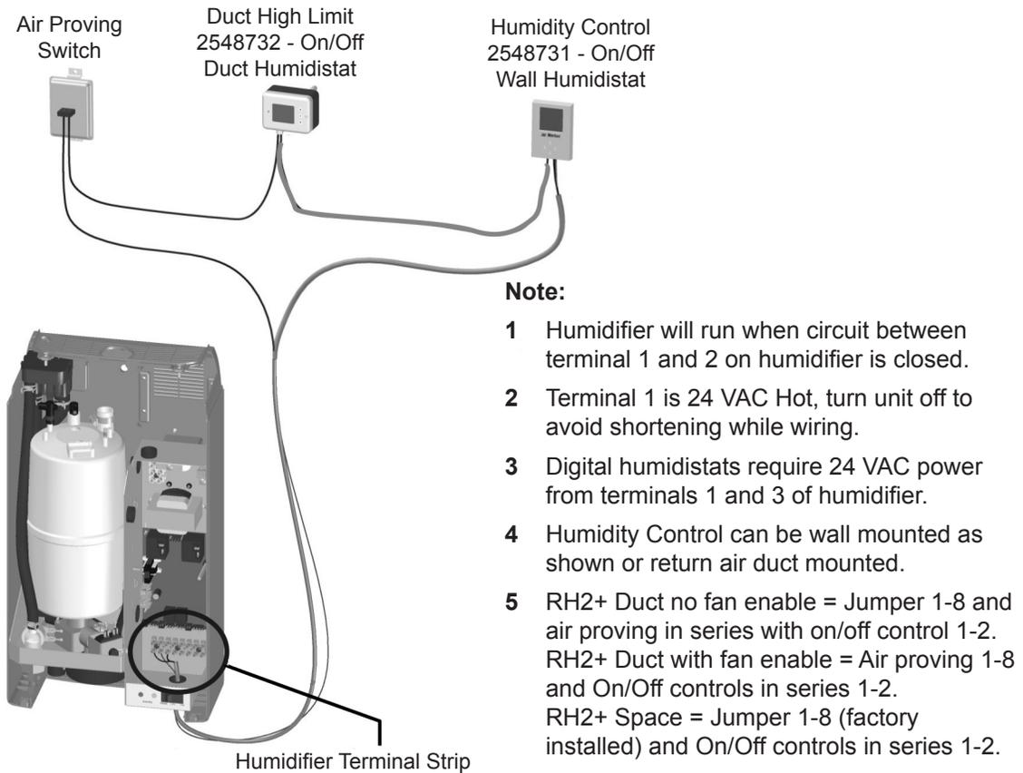
Figure 18: On/Off Controls
