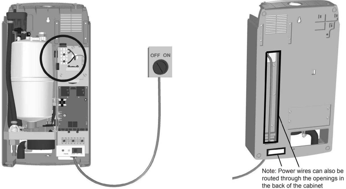
Note: Power wires can also be routed through the openings in the back of the cabinet
