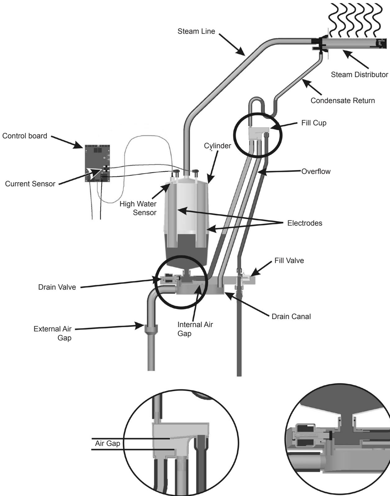
Figure 29: Humidifier Schematic
