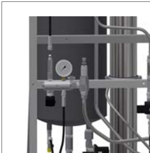
Fig. 26: Connecting HP discharge hose
