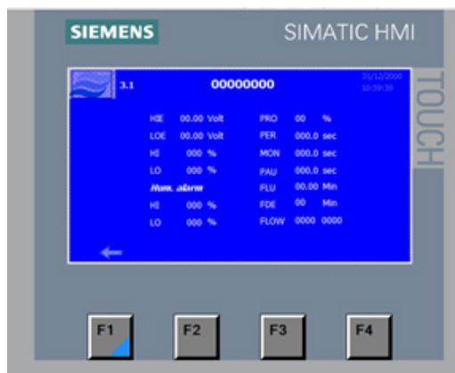
Display 3.1 - Zone controller
