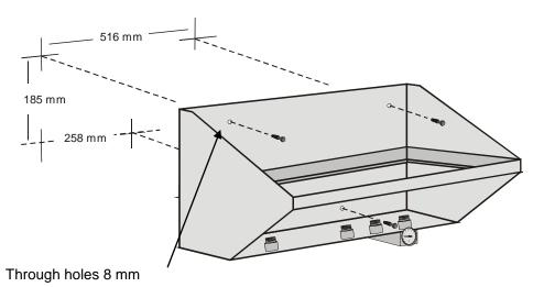
Figure 11: Hole pattern, support console
