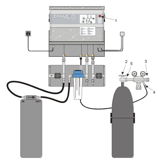
Figure 20: Replacing the CO<sub>2</sub> bottle
