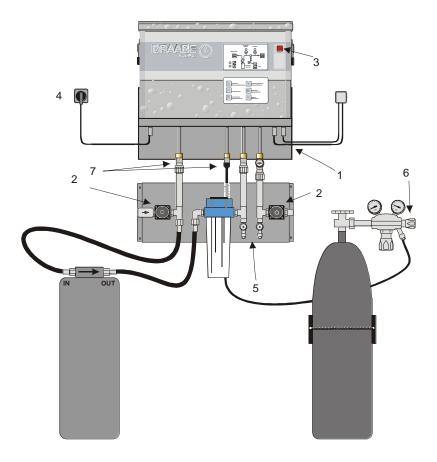
Figure 18: Replacing the SynPur
