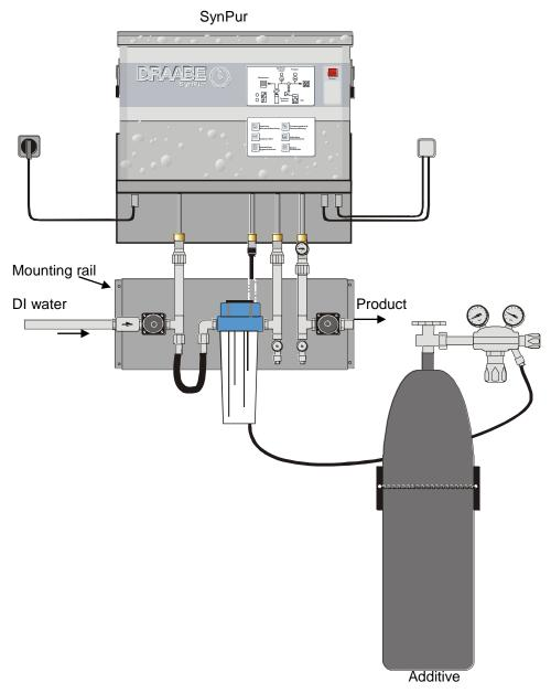
Figure 4: Conductivity Synthesizer with existing DI stage
