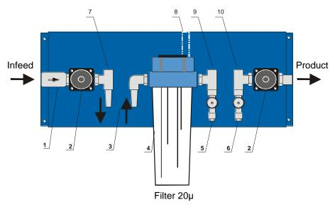
Figure 17: installation rail
