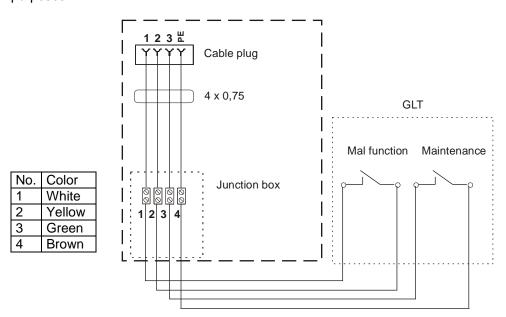
Figure 14: Linking to the GLT
