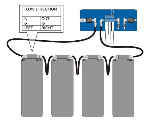
Figure 9: Sequential connection of synthesizer cartridges
