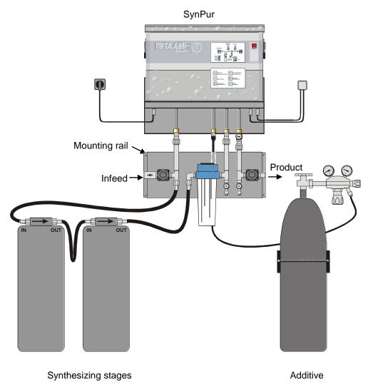
Figure 3: Basic System B with two synthesizing stages
