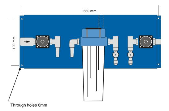
Figure 12: Hole pattern, mounting rail
