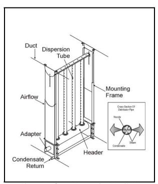
Figure 5. Short Absorption Manifold
