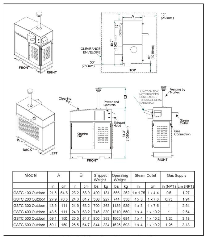
Figure 3. Physical Dimensions - GS Outdoor Humidifier
