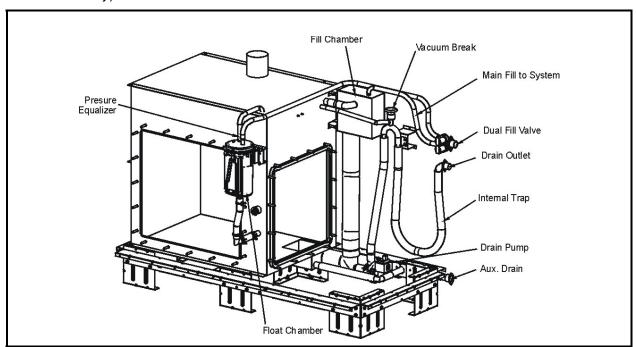
Figure 1. Humidifier Tank
