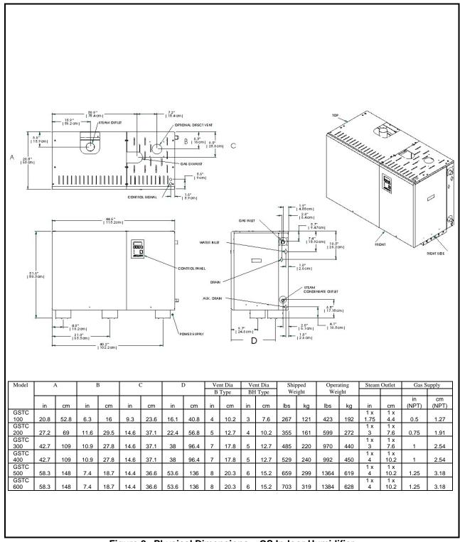
Figure 2. Physical Dimensions - GS Indoor Humidifier
