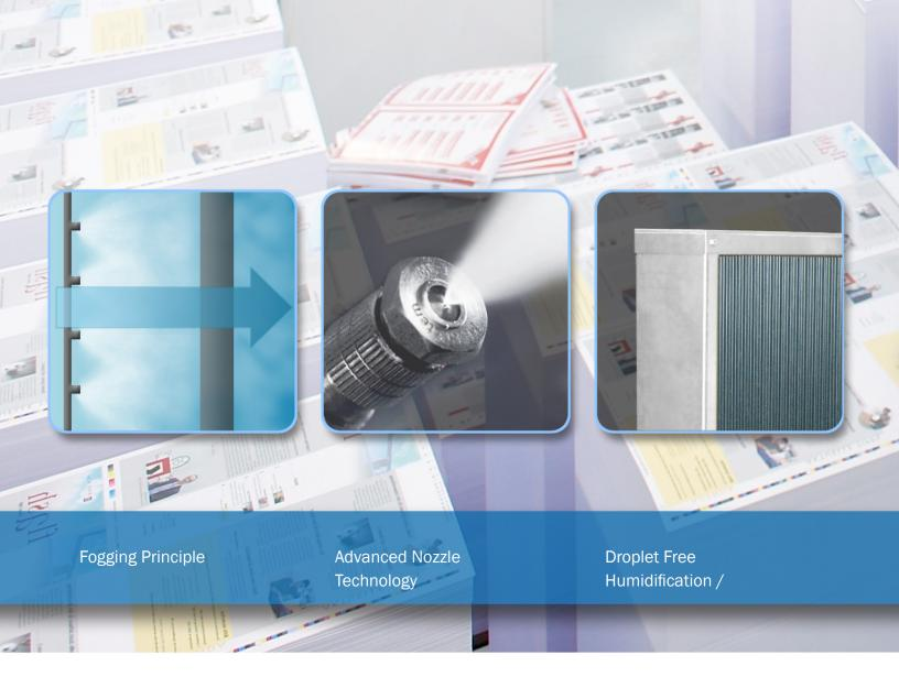
The Nortec HP-Series high pressure nozzle system supplies treated water at 1015 psi for installation in an air duct or air handler. Advanced atomizing nozzles generate a fine mist which is absorbed into the air stream while a highly efficient droplet separator contains any excess water within the spraying section. Cool, humidified air is then released into the air stream, creating a healthy and productive environment.
