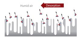
the silica gel and bind it as steam in the air (desorption). The now humid regeneration air leaves the adsorptiondryer and, if necessary after a supplementary heat recovery, is blown out to the outside air. Hot water, steam, gas burner or electrical energy are used as media for heating the regeneration air.
