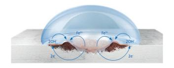
water, oxygen and hydroxide ions lead to ever more continuous reactions from which iron(III) oxide and iron(III) hydroxide are formed. These deposit on the metal surface and give the rust its typical appearance. In contrast to metals such as aluminum, the process is only stopped when iron is no longer present.
