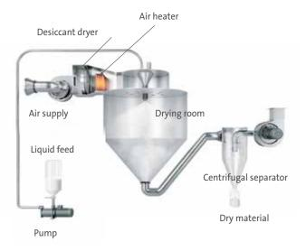
Adsorption dryers are ideally suited for the spray drying process. During the desiccant drying process, not only is the humidity of the process air reduced, but the air is also heated. This heating benefits the spray drying process, as heating the hot air requires large amounts of energy. This significantly improves the efficiency and cost-effectiveness of the spray drying process.
