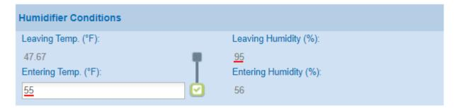
For agent selection the leaving humidity is restricted to <75% to reduce excessive waste water. The EAT will need to be increased to ensure the leaving humidity is <75%
