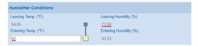
It is important that the EAT is not increased just to force the selection. That EAT is the new required temperature for the system and must match realistic conditions. A heating coil may be required.
