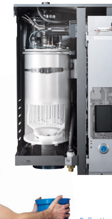
Collection tank is drained and emptied
