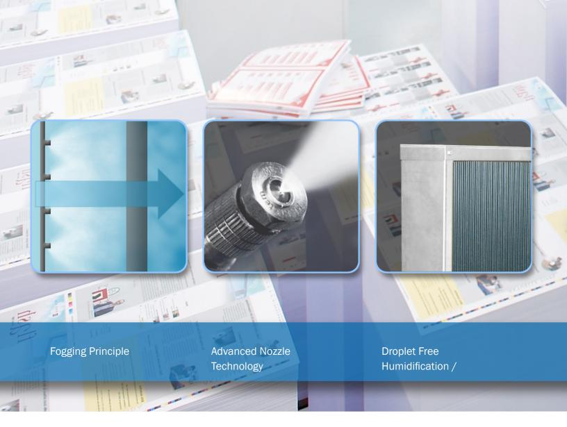
The Condair HP-Series high pressure nozzle system supplies treated water at 1015 psi for installation in an air duct or air handler. Advanced atomizing nozzles generate a fine mist which is absorbed into the air stream while a highly efficient droplet separator contains any excess water within the spraying section. Cool, humidified air is then released into the air stream, creating a healthy and productive environment.
