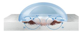
reactions from which iron(III) oxide and iron(III) hydroxide are formed. These deposit on the metal surface and give the rust its typical appearance. In contrast to metals such as aluminum, the process is only stopped when iron is no longer present.
