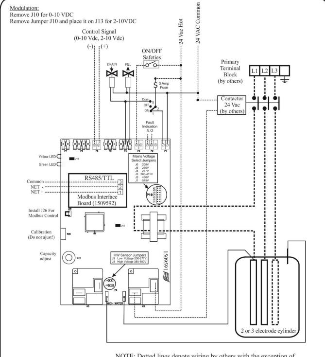
NOTE: Dotted lines denote wiring by others with the exception of Primary Voltage Wiring (PVW) units which will come with all primary wiring to the cylinder and 10' of wiring to run the electrical back to the contactor
