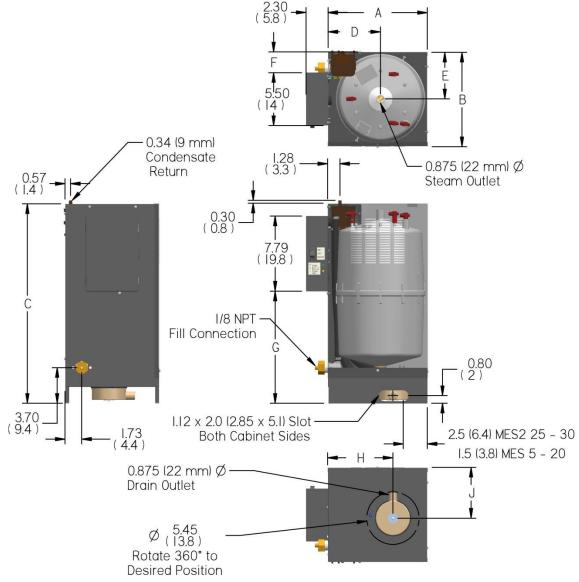
Note: Unless otherwise specified dimensions are in inches (cm). Tolerance ±0.1 in. (0.25 cm)
