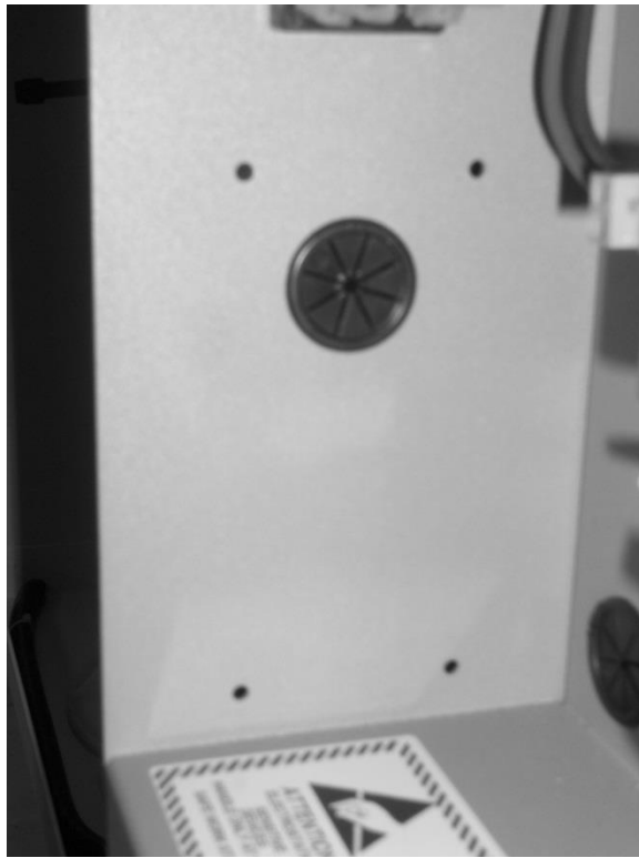
Figure 12: Pre drilled holes for Logic card
