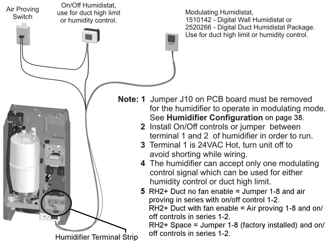
Figure 20: Modulating Controls
