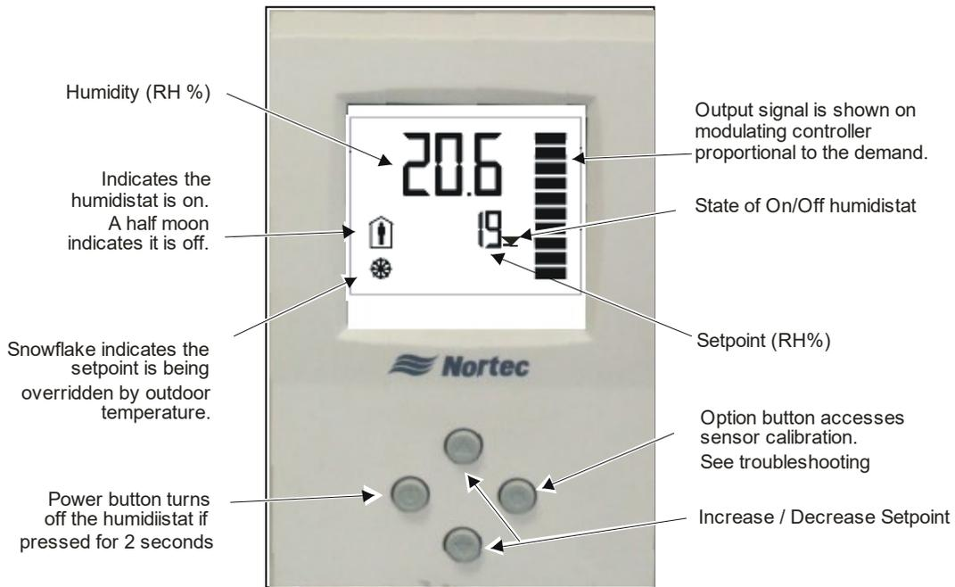
**Figure 26: Modulating and On/Off Digital Control Operation**
