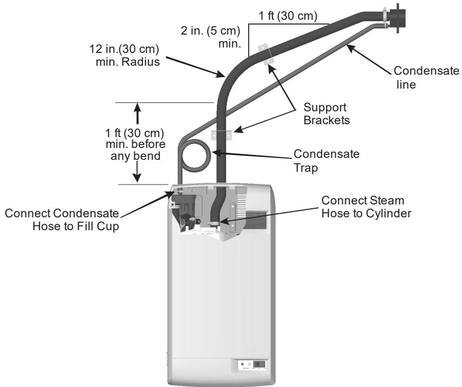
**Figure 11: Steam Distributor Above Humidifier (using Condair hose)**
