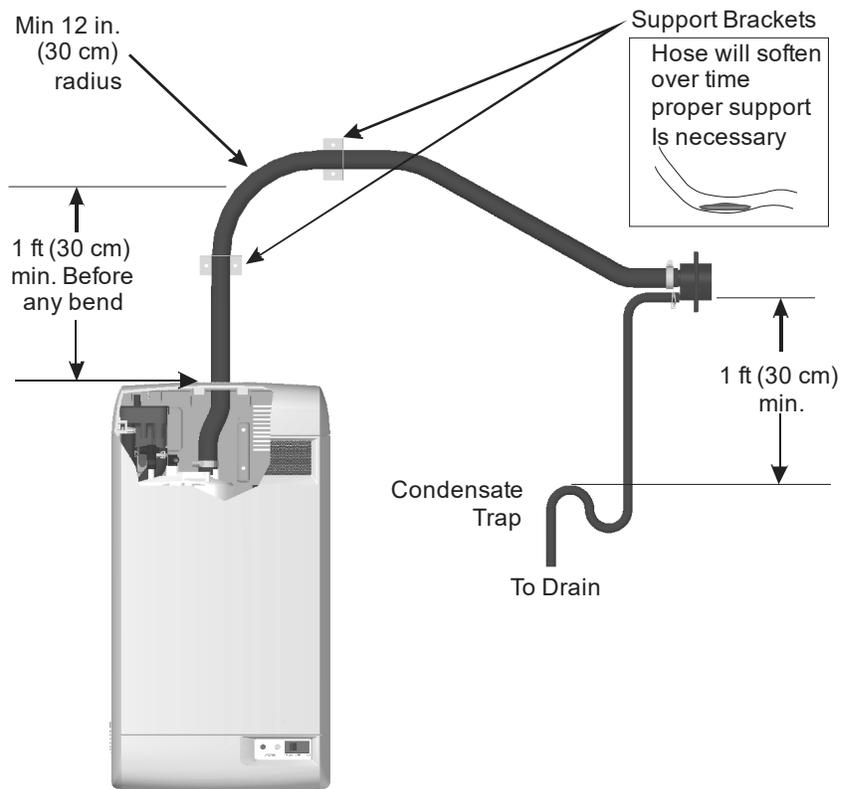
**Figure 12: Steam Distributor Below Humidifier (using Condair hose)**
