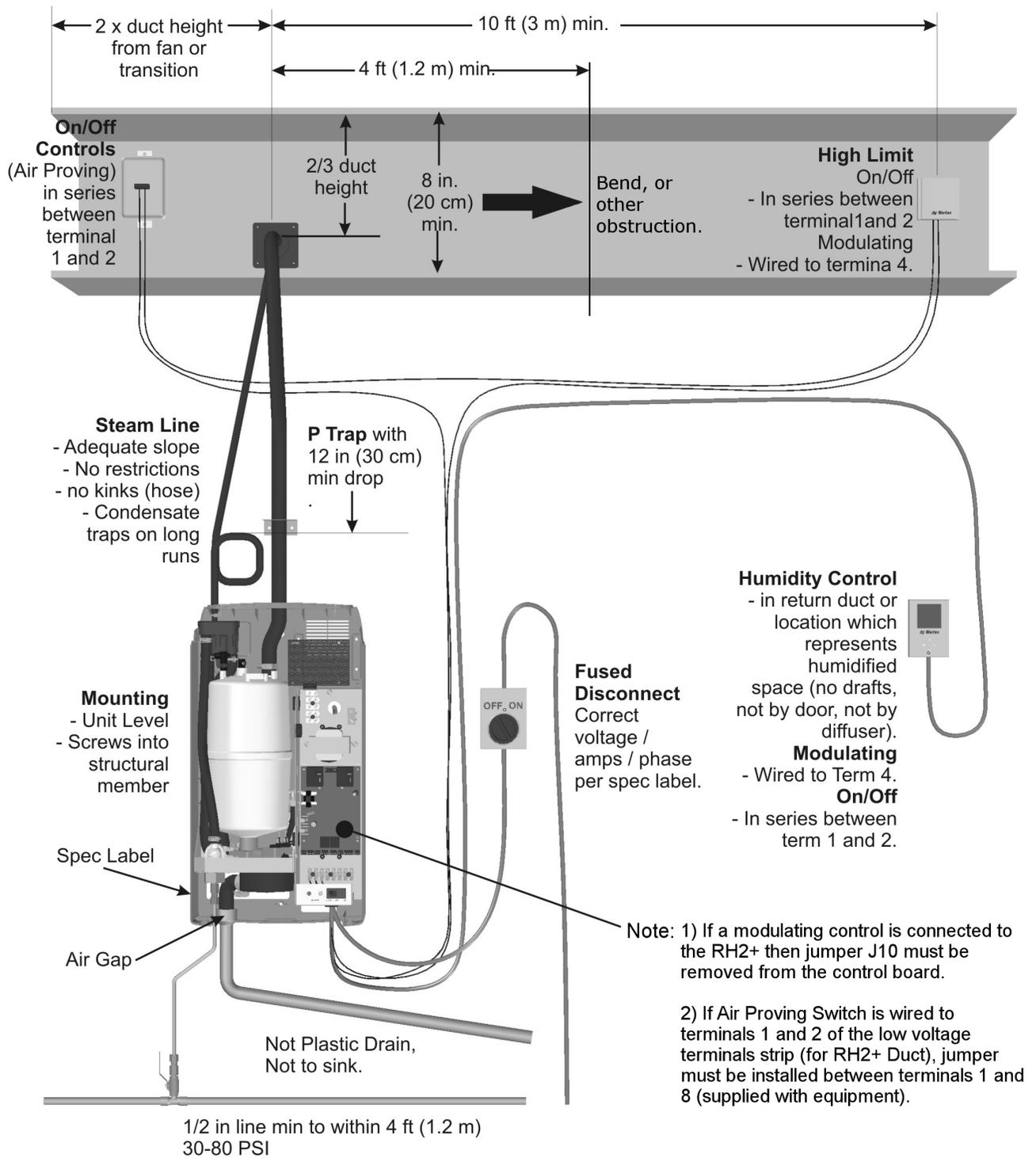
Figure 25: Installation Check
