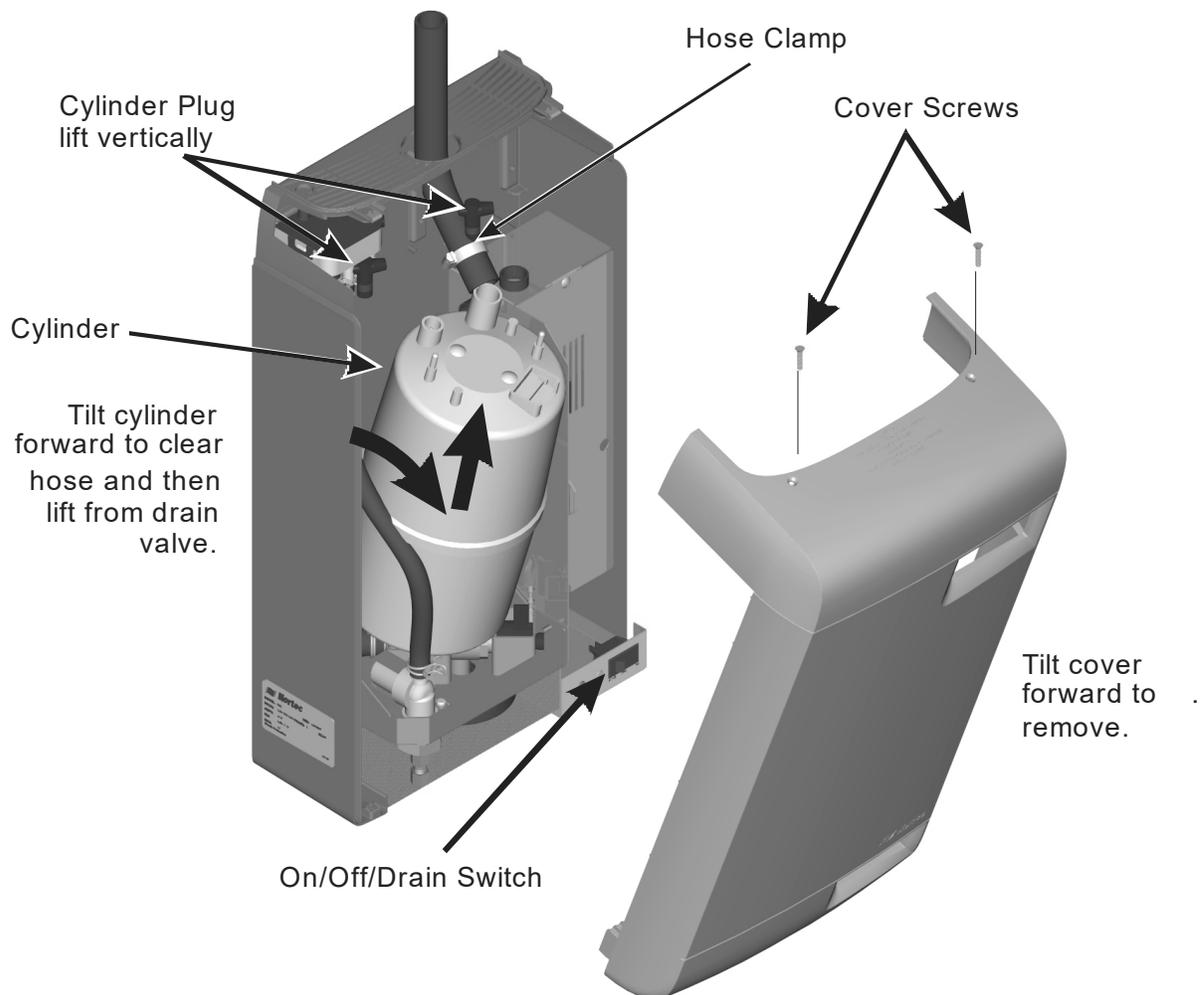
**Figure 34: Cylinder Removal**
