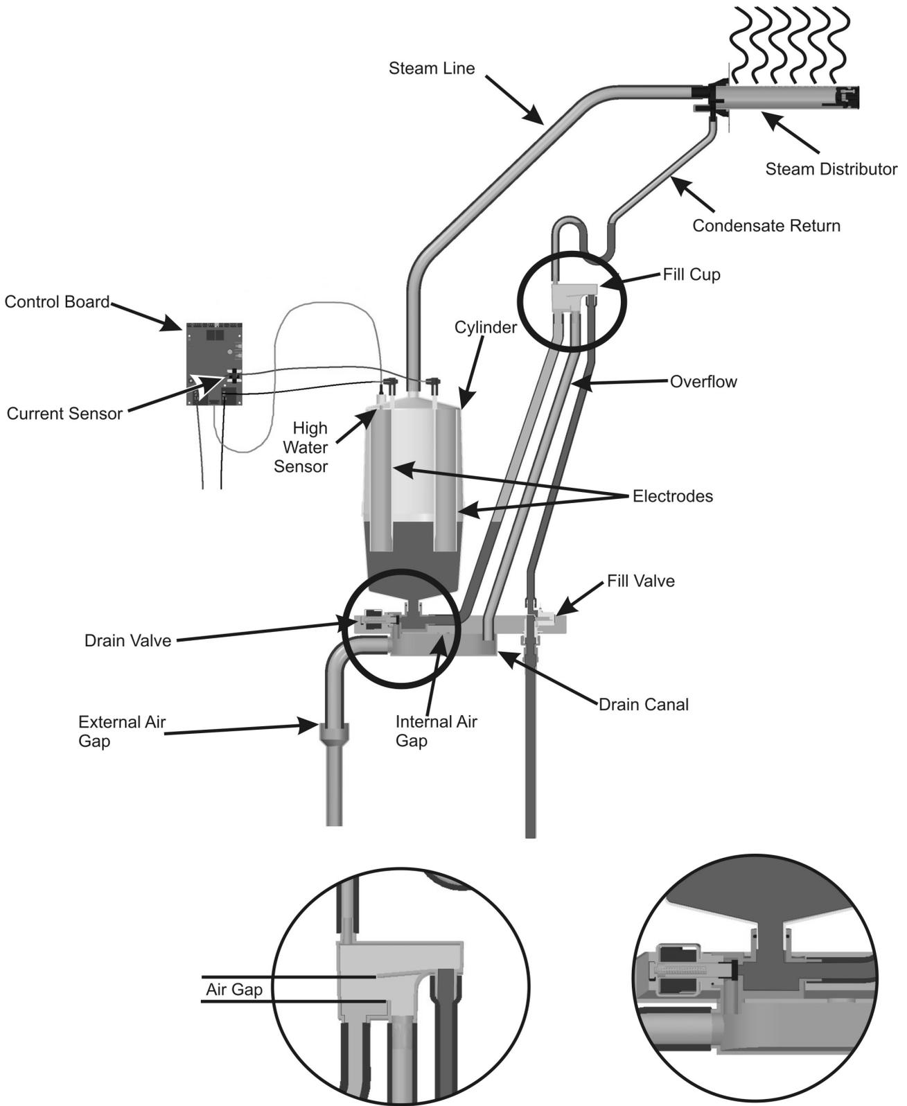
Figure 29: Humidifier Schematic
