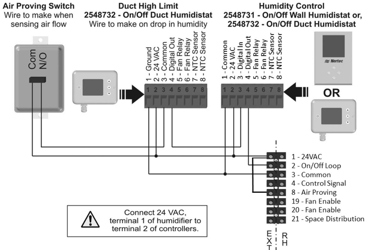
Figure 19: Digital On/Off Humidistat
