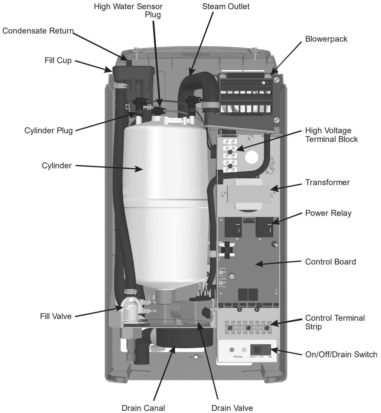
**Figure 28: RH2 Humidifier Components**
