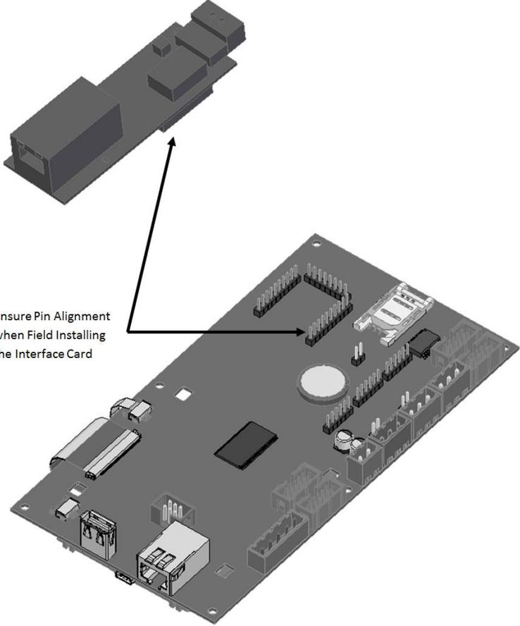
**Figure 6: Pin Alignment**
