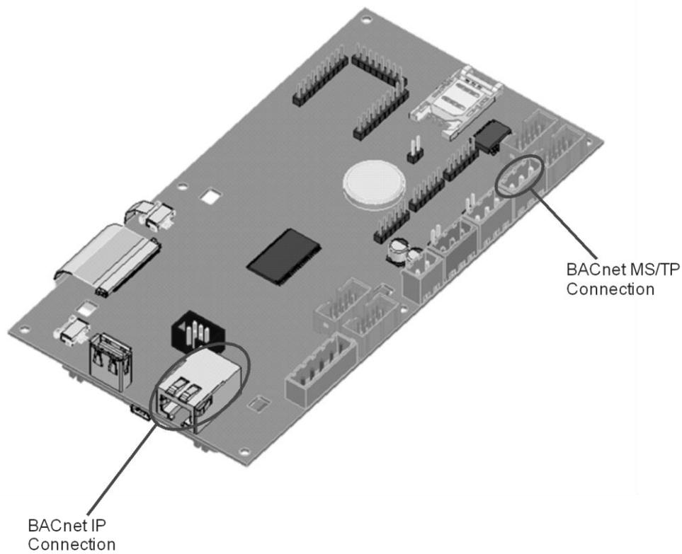
**Figure 2: BACnet MS/TP and IP Connection Location**
