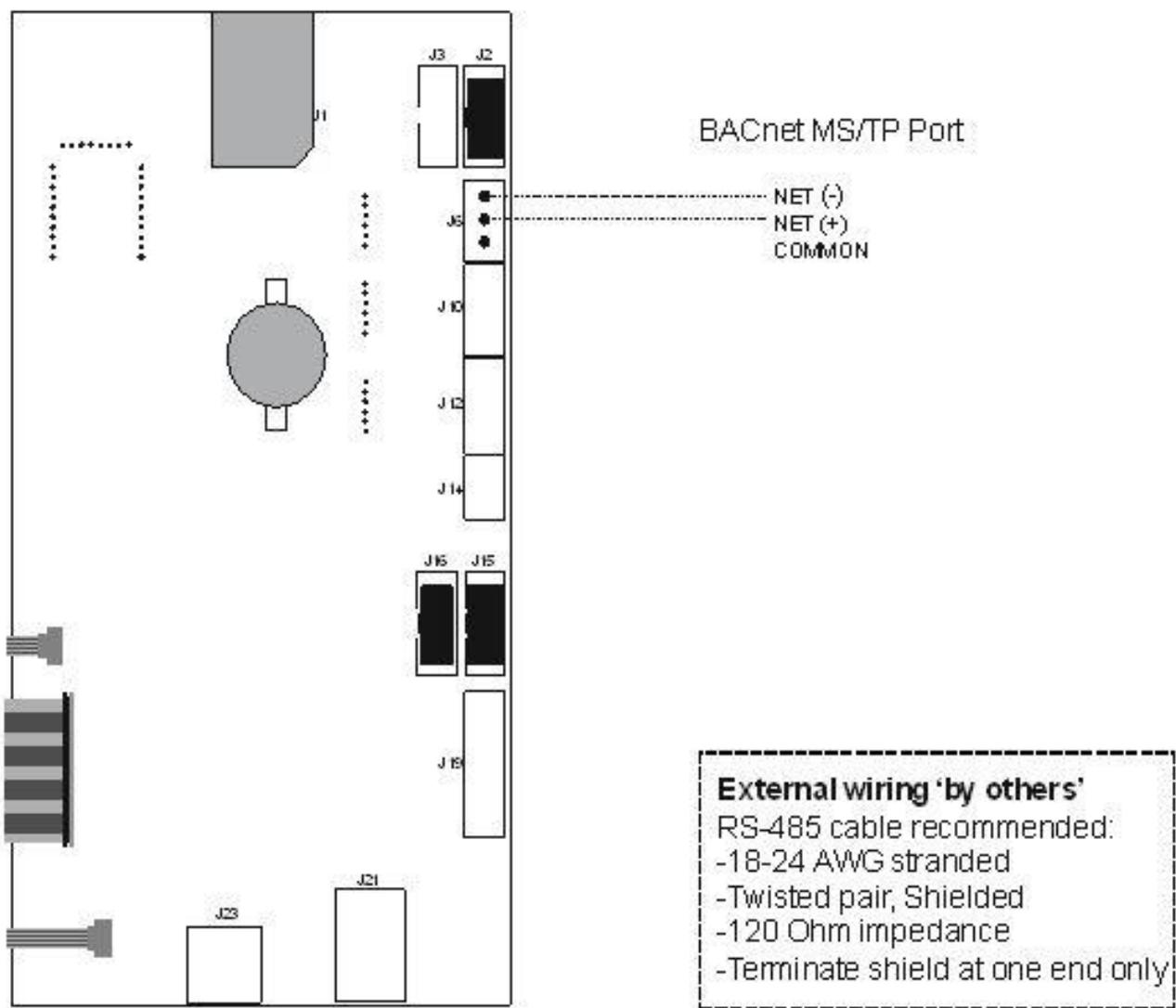
Figure 3: BACnet MS/TP Wiring Diagram
