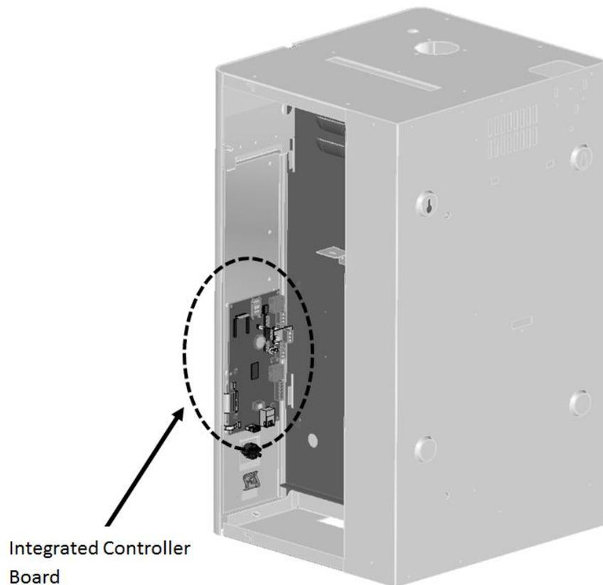
**Figure 1: Location of Integrated Controller Board**
