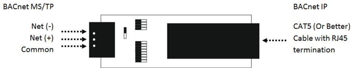
**Figure 8: BACnet Specific Ports**
