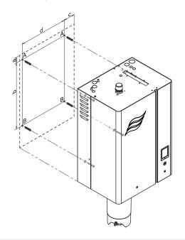
1. Mark the attachment points "A" and "B" at the desired position in the mounting surface with the help of a level.
