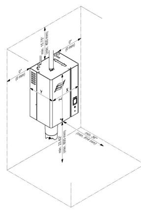
– Install the steam humidifier so that the minimum bend radius R=12" / 300mm for Condair hose, R=5 x internal diameter for hard pipes and upslope (min  $10^{\circ}$ ) / downslope (min  $2^{\circ}$ ) of the steam hose is maintained.
