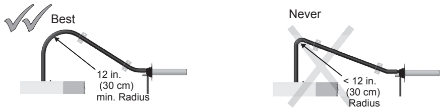
Figure 4: Minimum bend radius in steam lines.
