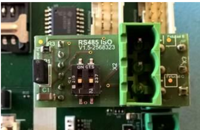
Fig. 4: Mounting the "Isolation Module" option
