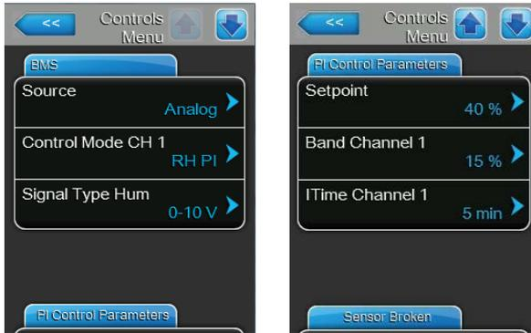
**"Source"** to **"Analog"**, **"Control Mode CH 1"** to **"RH PI"**, **"Signal Type Hum"** to **"0-10V"** (or to output signal set on CDC) or **"2-10V"** (for CDC-NA) and the parameters **"Setpoint"**, **"Band Channel 1"** and **"ITime Channel 1"** to the desired values (refer to the Condair DL operation manual).
