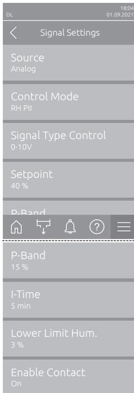
**"Source"** to **"Analog"**, **"Control Mode"** to **"RH PI"**, **"Signal Type Control"** to **"0-10V"** (or to output signal set on CRC) or **"2-10V"** (for CRC-NA) and the parameters **"Setpoint"**, **"P-Band"** and **"I-Time"** to the desired values (refer to the Condair DL II operation manual).
