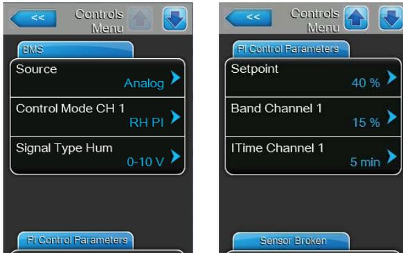
**"Source"** to **"Analog"**, **"Control Mode CH 1"** to **"RH PI"**, **"Signal Type Hum"** to **"0-10V"** (or to output signal set on CRC) or **"2-10V"** (for CRC-NA) and the parameters **"Setpoint"**, **"Band Channel 1"** and **"I Time Channel 1"** to the desired values (refer to the Condair DL operation manual).
