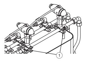
Gently rotate the whole pipe assembly by hand until the spray angle is nominally set. Retighten the pipe clamp fittings. The nozzles are now installed and you can move on to the next stage of the install and commissioning.
