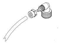
Slide the hose through the locking nut and fully over the stepped spigot of the fitting. It is a tight interference fit. Once the hose is in place refit the locking nut and tighten finger tight, then a 1/4 turn additional using a wrench.
