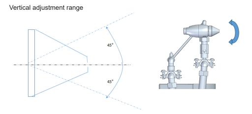
To adjust the verical angle of the nozzle, loosen the pipe clamp fixing screws (item 1), slightly on just the compressed air line.
