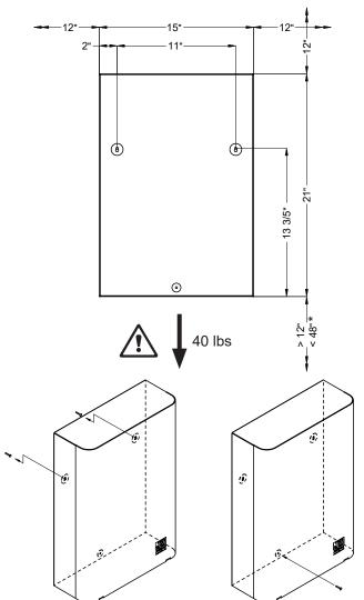
\*Recommended maximum installation height to allow service access without ladder or lift requirement.
