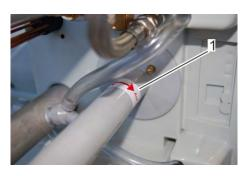
**6.** Loosen the water pump towards the right and pull out carefully (Fig. 47/1).
