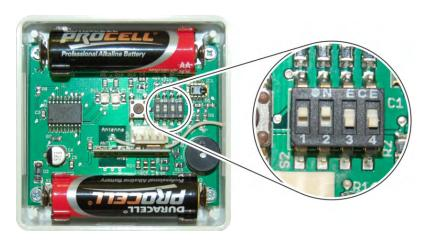
Fig. 15: Slide controls for coding
