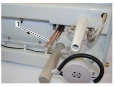
Fig. 26: Clean electrode rods
