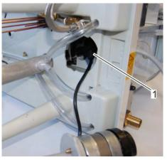
Fig. 48: Disconnect plug connection
