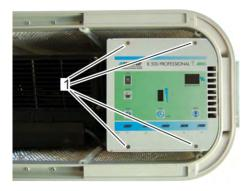
3. Use a screwdriver to loosen and unscrew the four screws at the surface of the control panel by turning counter-clockwise (Fig. 71/1).
