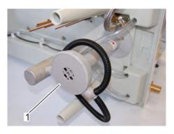
⇒ The water pump is located at the bottom on the right side (Fig. 45/1).
