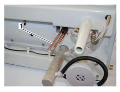
Fig. 41: Clean copper electrodes
