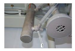
Fig. 67: Cleaning the stainless steel pipe
