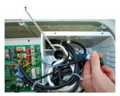
Fig. 73: Pulling out the UV lamp
