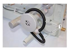
Fig. 50: Attach pump hoses
