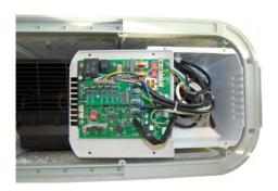
Fig. 20: Remove the control panel
