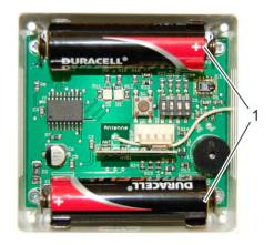
2. Insert the enclosed AA batteries according to the illustration (Fig. 12/1). The plus and minus poles are marked on the board as well as on the battery. The batteries are correctly inserted, if the markings match.
