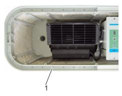
4. Check drainage holes of the water distribution (Fig. 24/1) for clogging. Remove residues such as lime or dust using a needle, a screwdriver or wet shop-vac.
