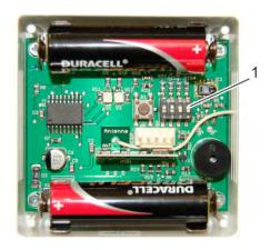
Fig. 17: Coding the wireless sensor system
