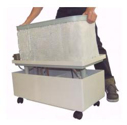
**3.** Lift center piece from the water tank and place on the side surface (Fig. 64).
