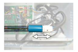
Fig. 74: Remove connection cable
