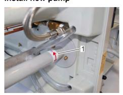
Fig. 49: Install pump
