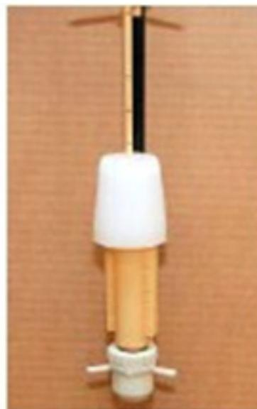
4. When installing the salt valve, be careful not to drop it down into the cylinder. If it is dropped, the float may sink and give an incorrect setting. Place the valve in such a way that the bent 3/8" pipe is placed along the back of the salt well away from the cylinder wall. Now press the 3/8" bent pipe into the notch, so that it extends 25 mm from the brine cylinder (see photo to the right).
