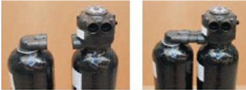
3. Fit the enclosed O-rings on the black plastic/brass connecting pieces and lubricate with silicone from the small tube. Then install the connecting pieces shown in the pictures below.
