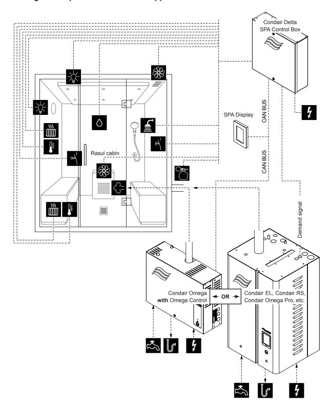
Fig. 6: Condair Delta SPA Control Box with equipment for Rasul application
