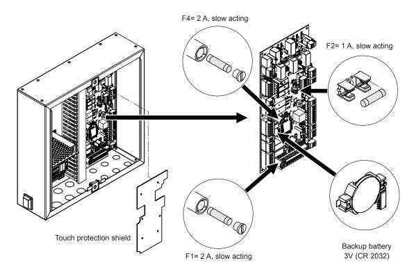
Fig. 7: Position of the backup battery and the fuses on the SPA control board
