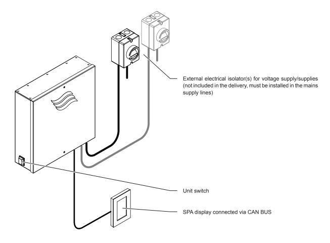
Fig. 2: Display and operating elements
