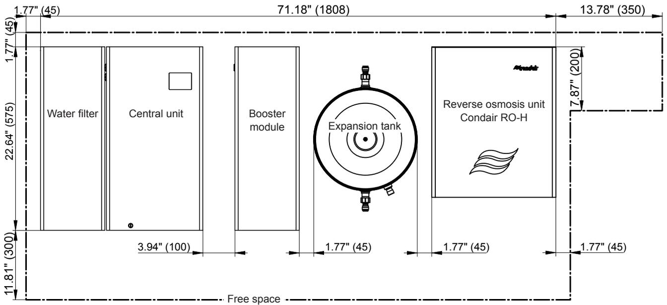
Fig. 13: Placement example 2 (dimensions in inch (mm))
