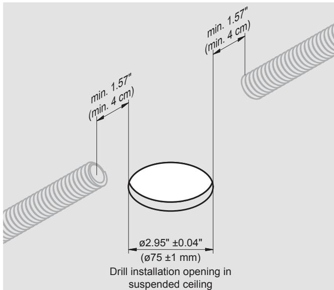
Fig. 21: Drill installation opening in the suspended ceilings
