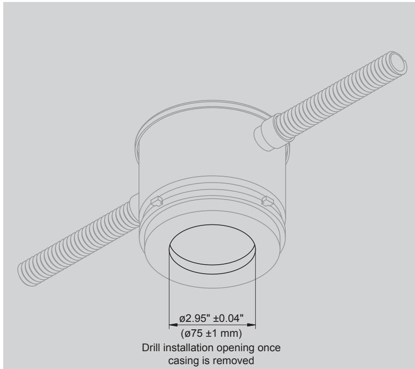
*Fig. 20: Drill installation hole in the installation box*
