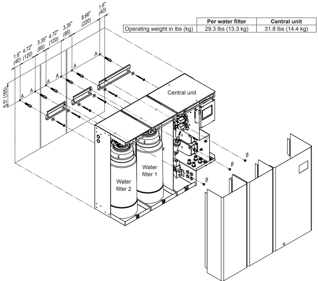
Fig. 24: Central unit installation overview (dimensions in inch (mm), illustration shows installation with screws and dowels)
