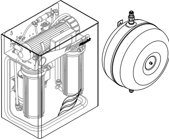
Reverse osmosis system RO-HB consisting of the reverse osmosis unit Condair RO-H and the 12 l expansion tank for feeding the central unit with RO water.
