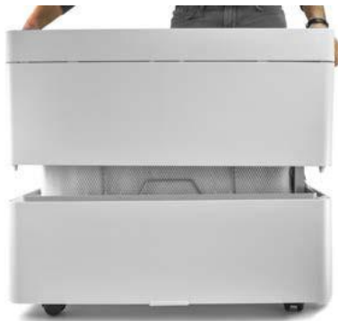
Fig. 4.3.1: Removing the upper part of the housing
