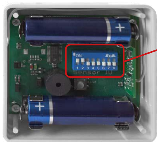
Fig. 5.6.1: Interior view of radio humidity transmitter
