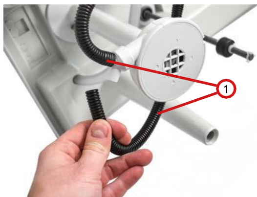
Fig. 6.3.4.4: Pulling off the pump hoses
