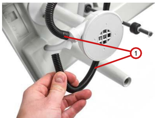
Fig. 6.3.4.4: Pulling off the pump hoses
