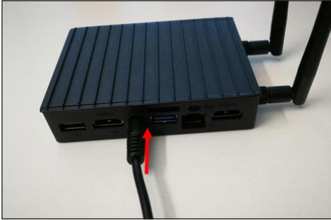
*Fig. 58: Connecting the gateway to the power supply*
