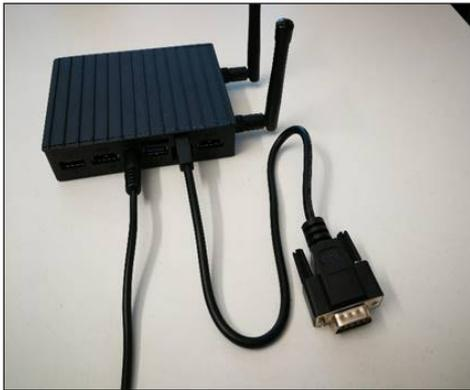
*Fig. 62: Connecting the gateway to the laptop using the RS232 cable*
