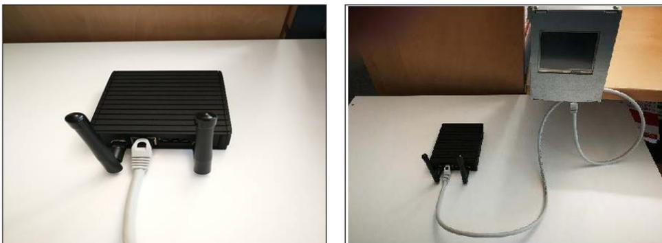
*Fig. 63: Connecting the gateway to the ConBox*
