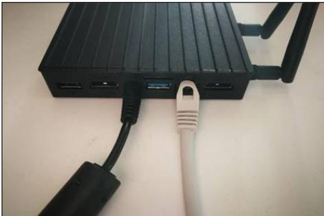
*Fig. 59: Connecting the gateway to the in-house network*
