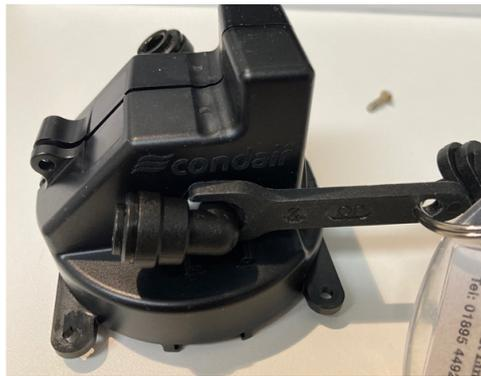
Remove the JG elbow on the screw head side.
