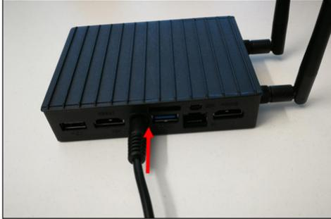
*Fig. 61: Connecting the gateway to the power supply*
