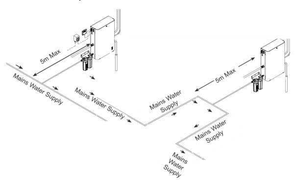
Stagnant water rapidly deteriorates in quality; it is therefore important that supply pipework and uncommissioned units are not filled with water and then left to stand in a wet condition. Even when drained pockets of moisture tend to be left behind, see the next section on commissioning.
