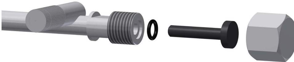
Fig. 29: Plugging pipe ends
