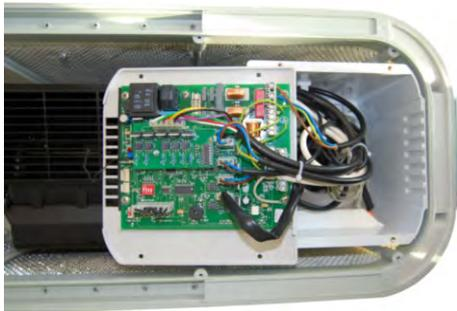
*Fig. 20: Remove the control panel*
