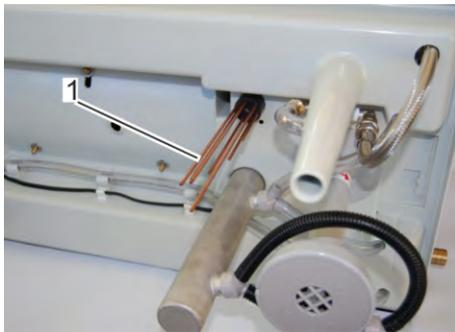
*Fig. 41: Clean copper electrodes*
