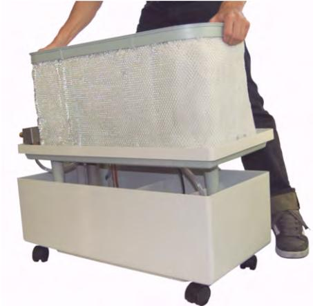
Fig. 64: Remove center piece
