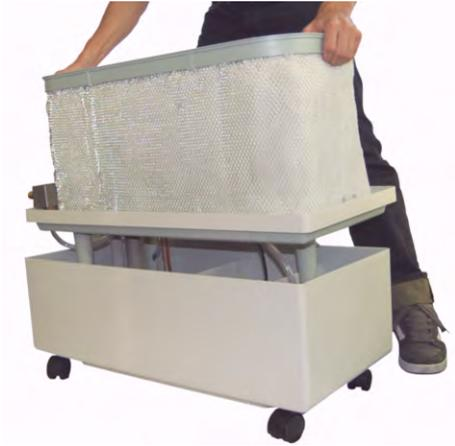
Fig. 53: Remove center piece
