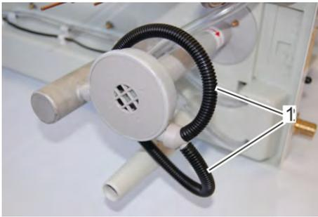
Fig. 50: Attach pump hoses
