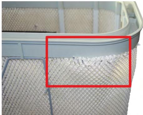
Fig. 10: Wrong fit of filter
