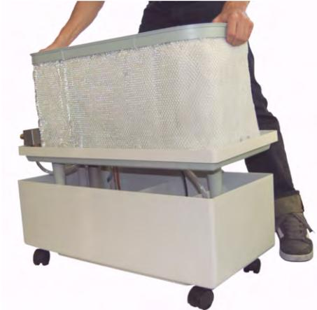
Fig. 44: Remove center piece
