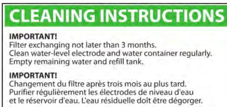
The sign at the filling opening provides important instructions for cleaning and care of the humidifier. For detailed instructions on cleaning and care of the humidifier heed [Chapter 6](#) "Cleaning and servicing the humidifier" on page 43.
