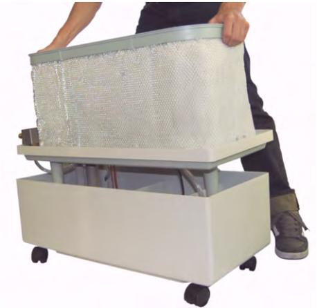
Fig. 25: Remove center piece
